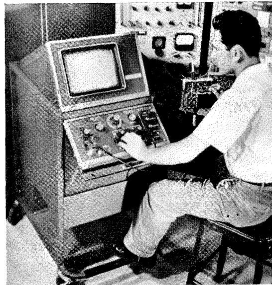
Figure 10—Precision oscilloscope using 14-inch (36-centimeter) cathode-ray tube.
