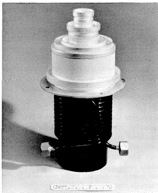
Figure 5—Ceramic-insulated triode for radio-frequency heating produces full output of 24 kilowatts at 100 megacycles per second.
